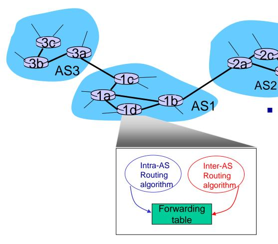
forwarding table configured by both intraand inter-AS routing algorithm
