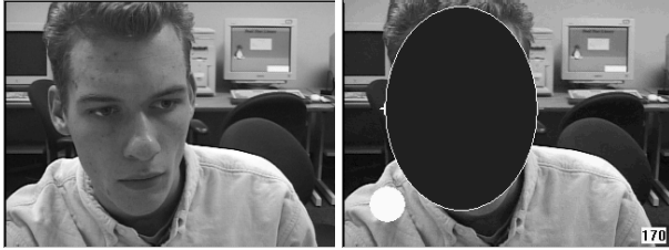
Figure 6: The face in the left image is detected and modeled by the ellipse shown in the right image.
