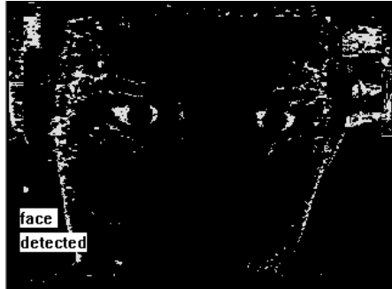
Figure 3: Pixels that match the sclera color are shown in white; other pixels are shown in black.
