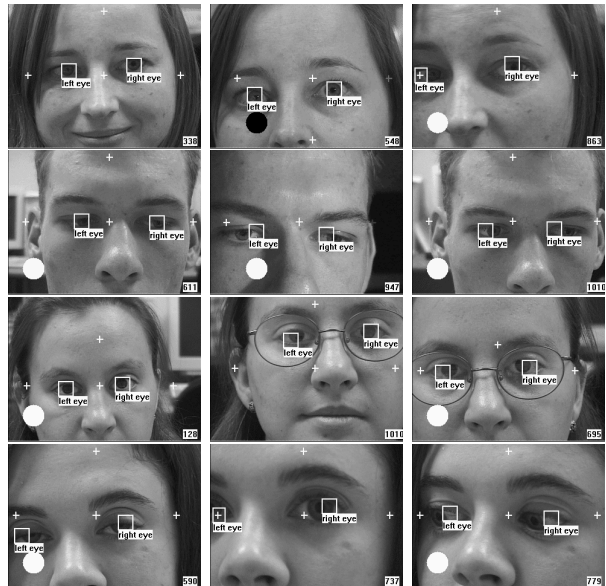
Figure 8: Eye detection and iris localization.
