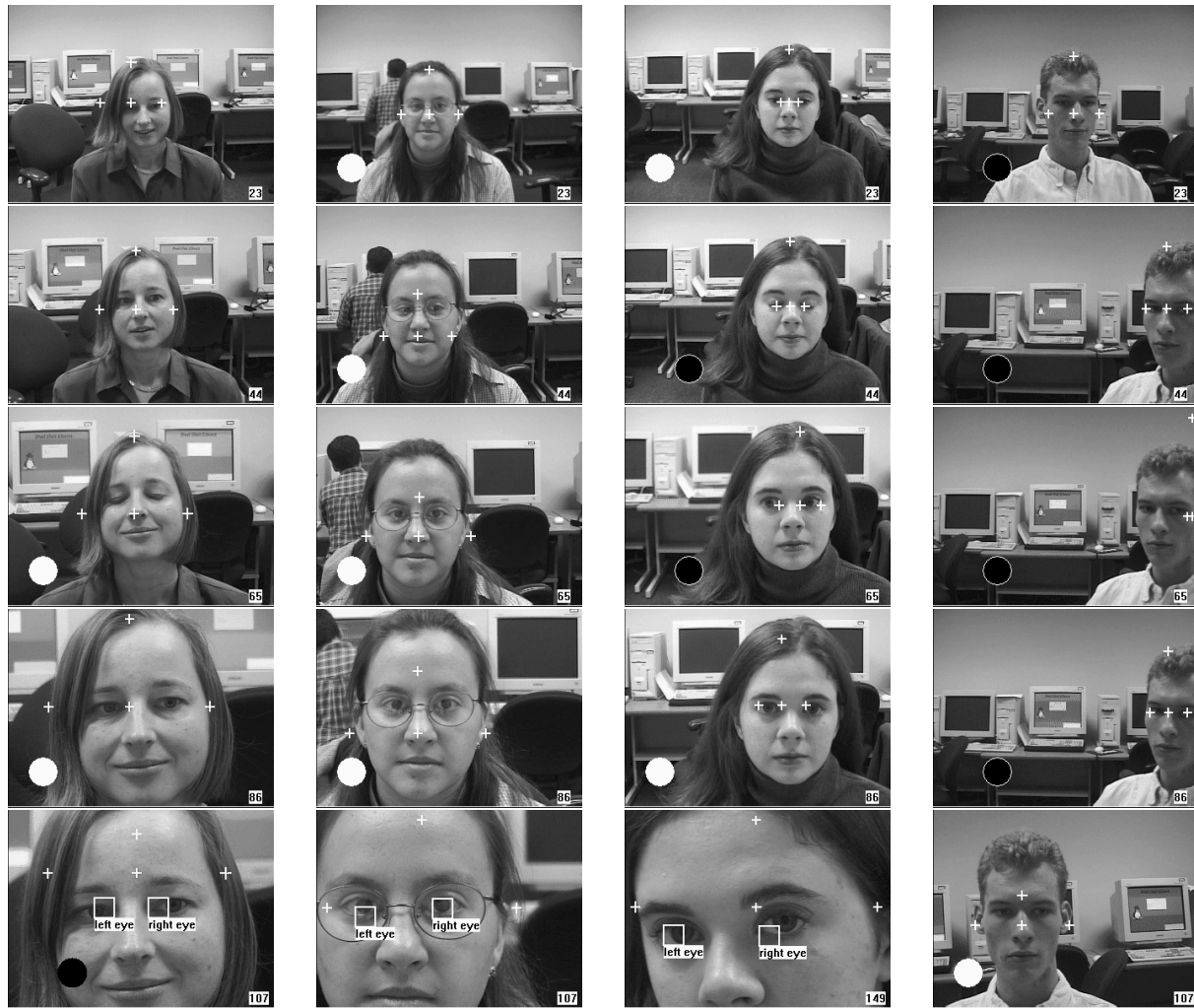
Figure 7: Once a face is detected, the system rotates to center the face within the image frame and widens the field of view. The faces detected in frame 23 have a width of about 55 pixels. Eye detection starts once the width of the imaged face is 231 pixels.
