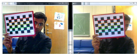
Fig. 2. A screenshot of the Multi Camera Capture system while it is used to record images simultaneously from two cameras in an experiment. In the field of view of the two cameras is a board with a checker pattern, which is used for spatial calibration of the cameras.
