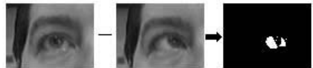
Figure 2: Motion detected by frame differencing is thresholded and used as a mask for the left-right image differencing.
